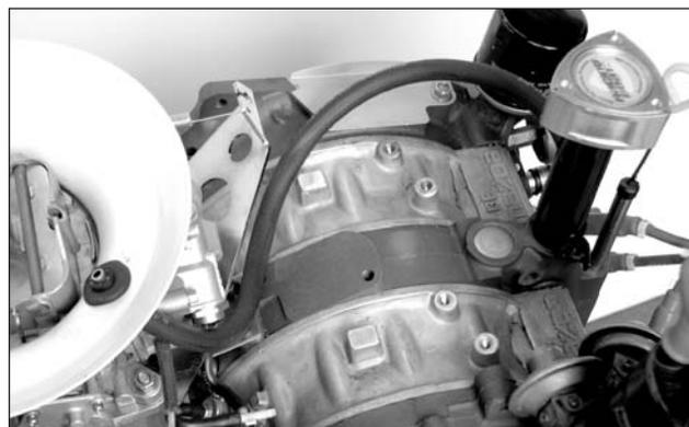
**Photo 10 - Connect the hose from the air filter to the air-oil separator.**
