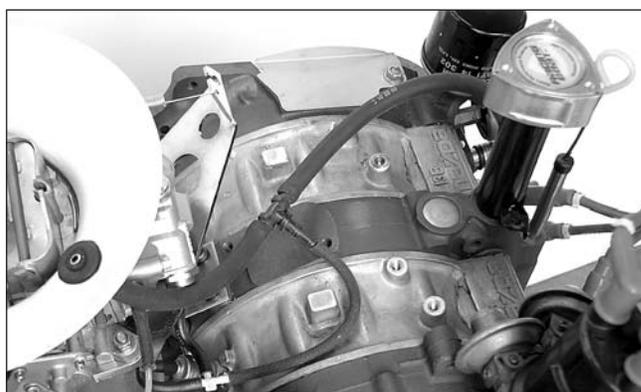
**Photo 11 - Cut the hose and install a plastic "T", complete the connection to the metering oil injectors.**
